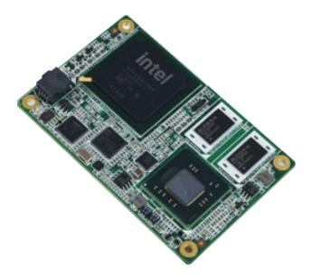
The SOM-7562 COM Module will soon be available with the option of an Intel® Atom™ N455 1.66 GHz CPU that supports ultra-fast DDR3 memory.
